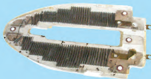
Fig. 10.11 Element of electric iron
