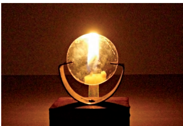
Fig. 11.26 Virtual image formed by the convex lens
