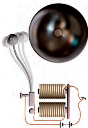
Fig. 10. 20 Circuit of an electric bell
