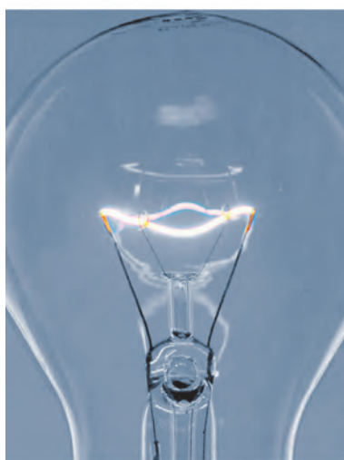
Fig. 10.12 Glowing filament of an electric bulb (incandescent)
