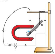
**Procedure:** 1. Take a small aluminium rod AB (of about 5 cm). Using two connecting wires suspend it horizontally from a stand, as shown in Fig.
