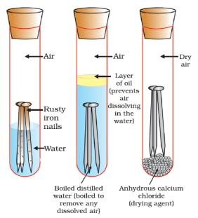
**Procedure:** i) Take three test tubes and place clean iron nails in each of them.
